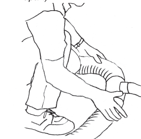
Push fit 'T' piece in ducting
